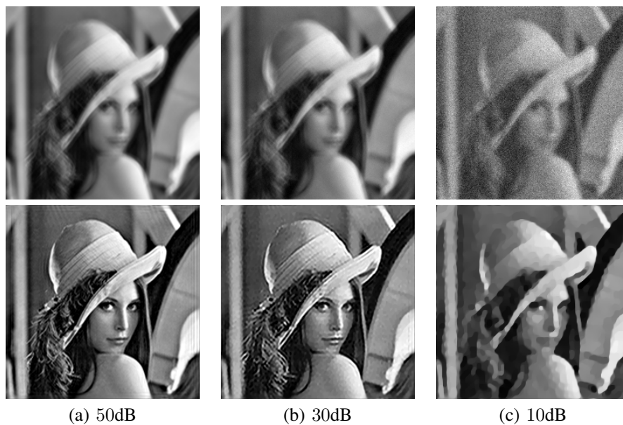
Fig. 11. Estimated sharp images for the PSF size set to 21 \times 21 and three different noise levels: (a) 50dB, (b) 30dB, (c) 10dB. Results are arranged as in Fig. 10. The first row shows one of the input images and the second row shows the estimated image.
