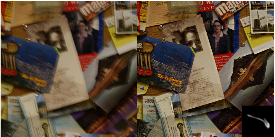
Fig. 4. Deconvolution of true motion blur. Left: captured image, right: deconvolved result (estimated PSF superimposed).
