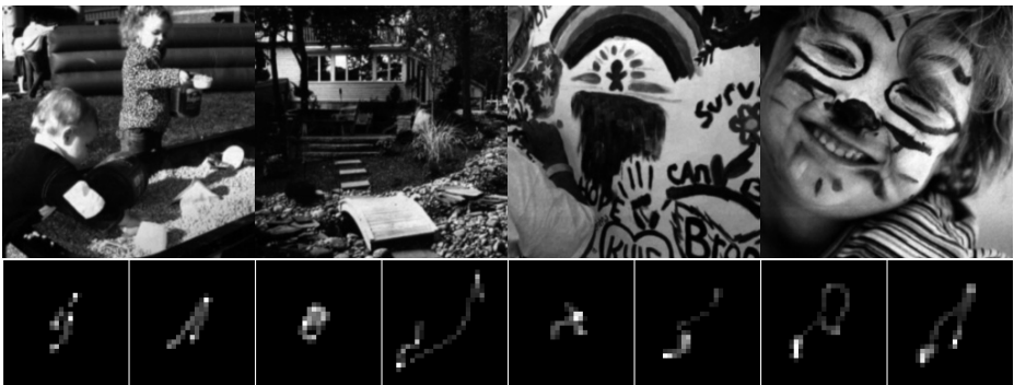
Fig. 1. The dataset of [10]. First row contains sharp images, second row measured motion blur PSFs.
